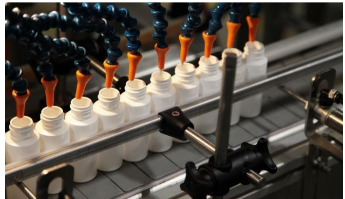
Close-up of the 10 head filling system
