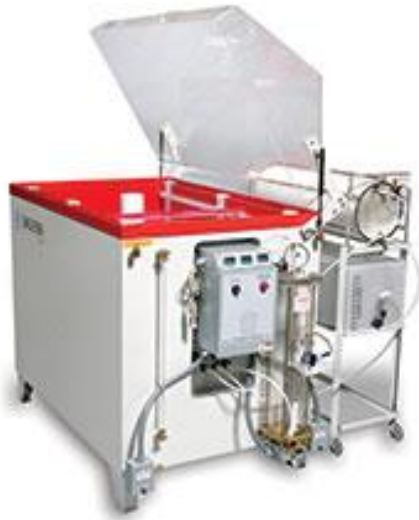
Accelerated Corrosion Test 1,000 hours SO 2 Salt Fog, ASTM G85 Annex 4 (24 Test Vehicles) Lockheed Martin
