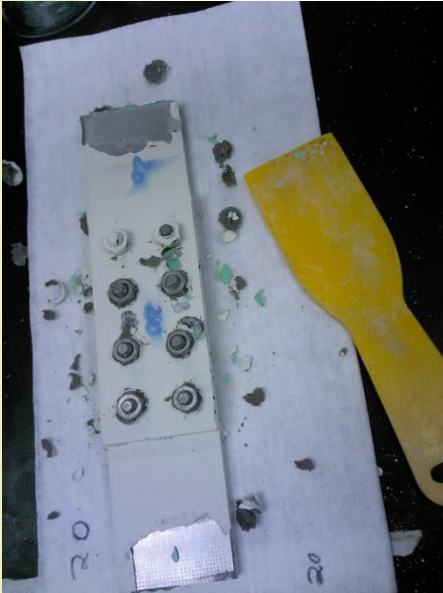
Sealant Removal TURI, UMass Lowell
