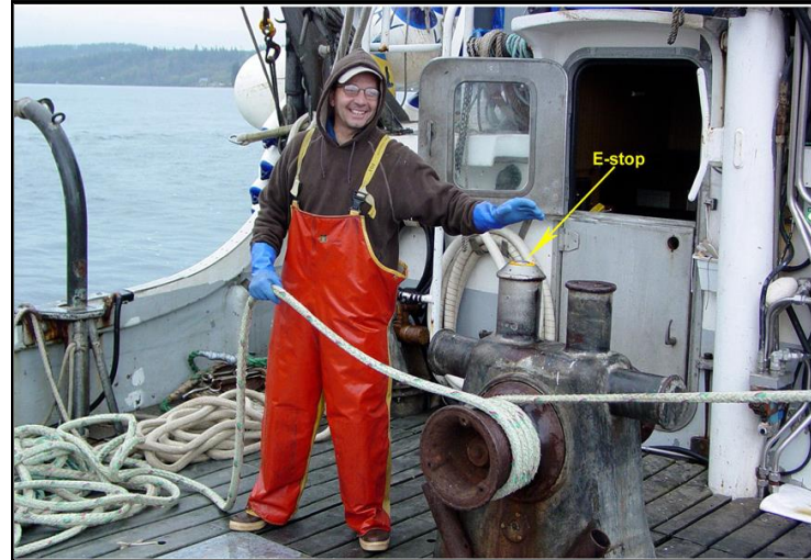
A fishing vessel captain demonstrating the use of an emergency-stop (e-stop) mounted on the winch
