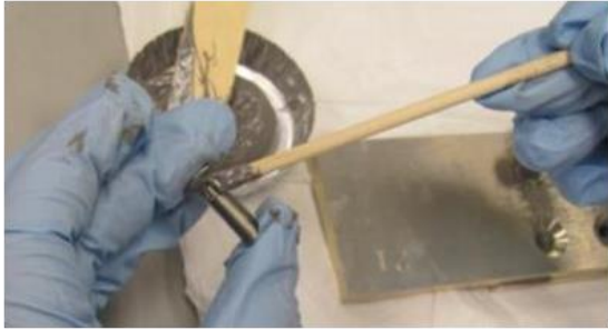
FIGURE 6.4.3 SEALANT BRUSHED ON TO FASTENERS
