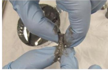
FIGURE 6.4.3 SEALANT BRUSHED ON TO FASTENERS
