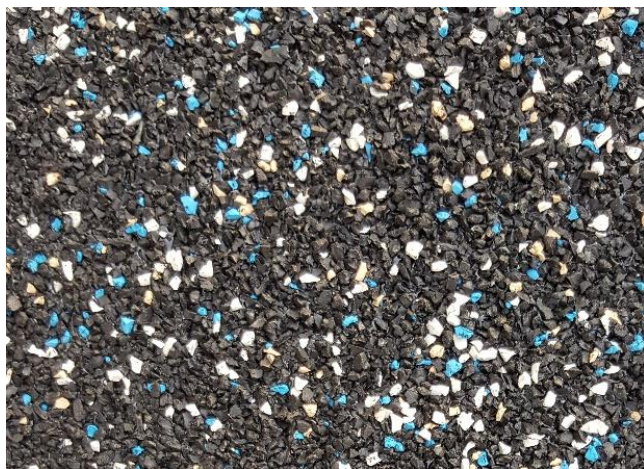
PIP consists of EPDM, TPE, or waste tire granules, held in place with adhesives.
