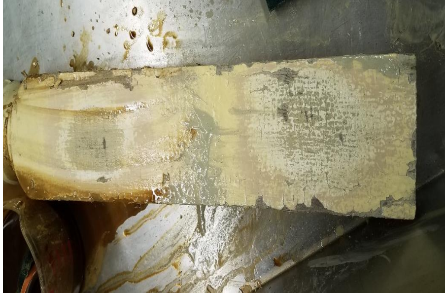
Figure 6: Testing results after 34 minutes (B7 on left side, Formulation #4 on right side)
