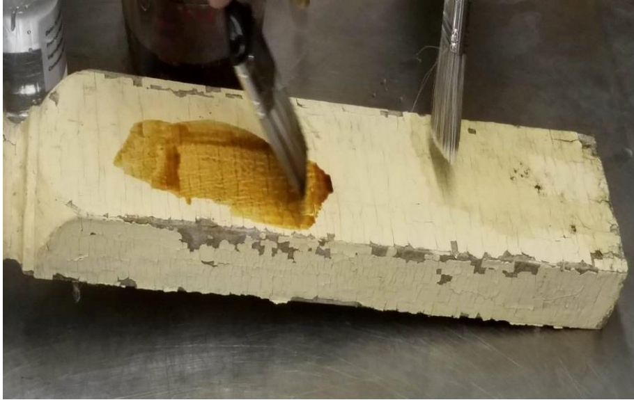
Figure 3: Initial application of paint stripping materials (B7 on left side, Formulation #4 on right side)
