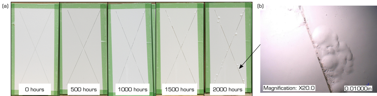
Figure 4. Neutral salt fog results on painted coupons for PPG RW-5562 on 2024 aluminum alloy test panels.
