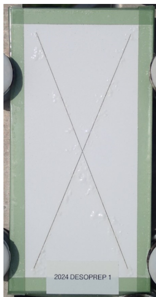
Figure 6. DESOPREP™ 4000 on 2024 alloy test panel #1 after nine months beachfront exposure.
