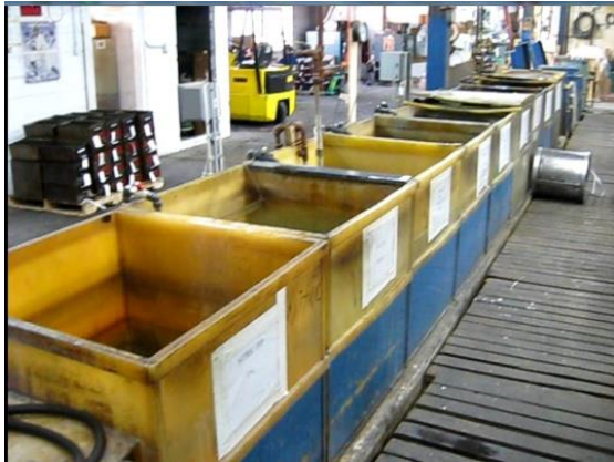
Conversion Coating MIL-DTL5541 (MacDermid Iridite 14-2) Northrop Grumman Maryland
