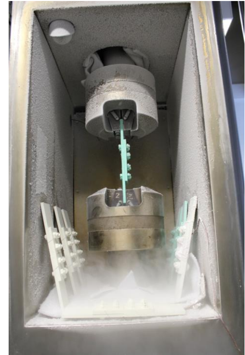
Thermal and Mechanical Preconditioning (MIL-PRF-81733D, Section 4.8.9.3.1 Cyclic Loading for Class 1 Materials) U.S. Navy – NAVAIR Maryland
