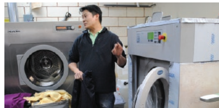
Joon Han of AB Cleaners demonstrates professional wet cleaning technologies, a safer replacement to dry cleaning machines that use perchloroethylene.
